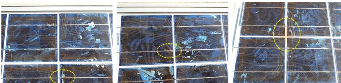
Figure 5: Examples of degradation and faults identified or suspected during visual inspection, for the case of p-Si modules.
