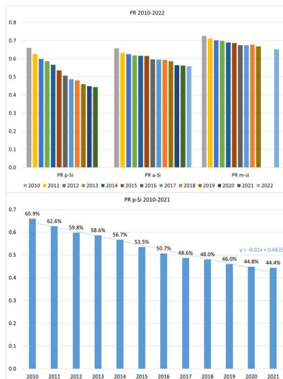
Figure 2: Top: Evolution of PR for the studied modules (2010–2022). Bottom: PR decrease for the p-Si modules for the same period.).
